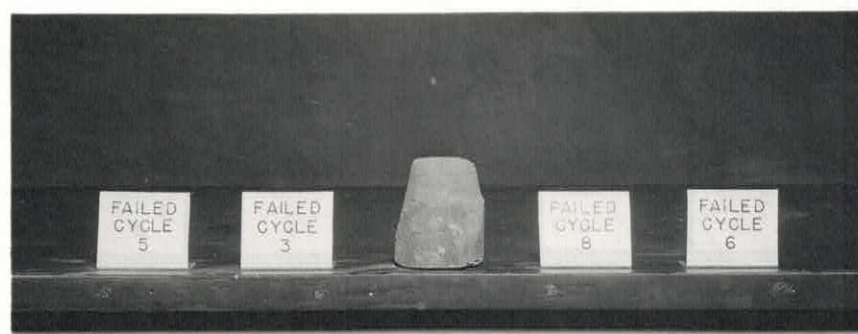
Brushed Specimens After Cycles of Freezing and Thawing
