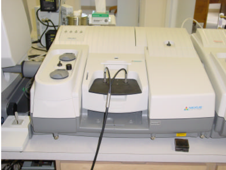
Figure 2-1. Nicolet 670 FT-IR Spectrometer with fiber port probe installation.
