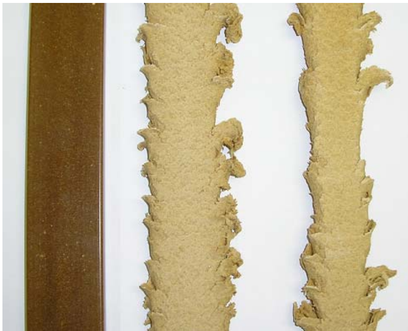
Figure 2.5. Extruded TPER/WF composites containing 2% OPE629A, 1% OPE629A, and 3% WP2200 from left to right, respectively.
