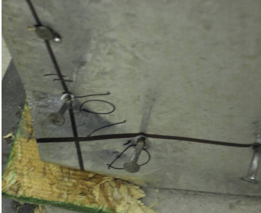
Figure 3.9 Buckling of metal gusset plate and damage of OSB at corner of wall
