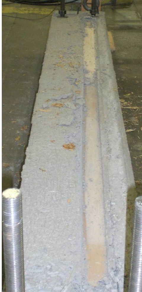
Figure 3.11 Failure of the first continuously embedded wall. Light colored area is WPC failure and the dark colored area is melt bond failure.
