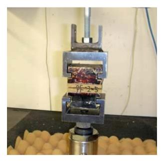
A piece of straw fiberboard undergoes the internal bond strength test for Laborie's project.
